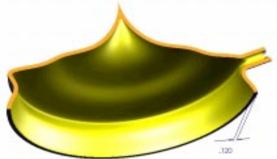
Figure 7. Test 7 focuses on the ability of solid modelers to develop complex revolved shapes from non-analytic curves (splines).
